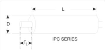
IPC SERIES epoxy casted mica capacitor, especially designed for PLC and high voltage application circuitry to extract HF signal from LF HV transmission line. It can also be used in very high voltage circuit. Utmost care has been taken in every s tep of manufacturing process covering with high withstanding voltage capabilities of dielectric..
